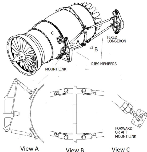
FIGURE 2 Detail configuration of QEC engine mount
