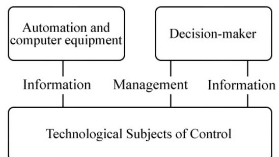
FIGURE 1 The structure of centralized APCS
